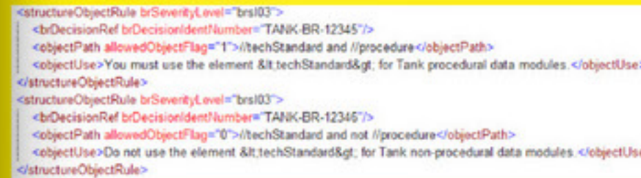
FIGURE 5 - EXAMPLE: CHECKING THAT <TECHSTANDARD> IS ONLY USED IN PROCEDURAL DATA MODULES
