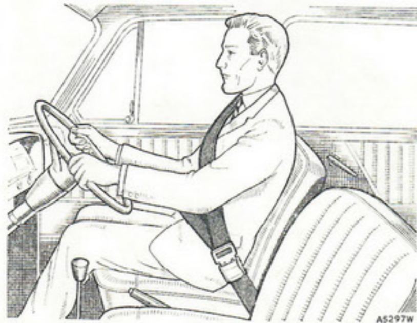
The seat belts in use, showing the correct position of the buckle
